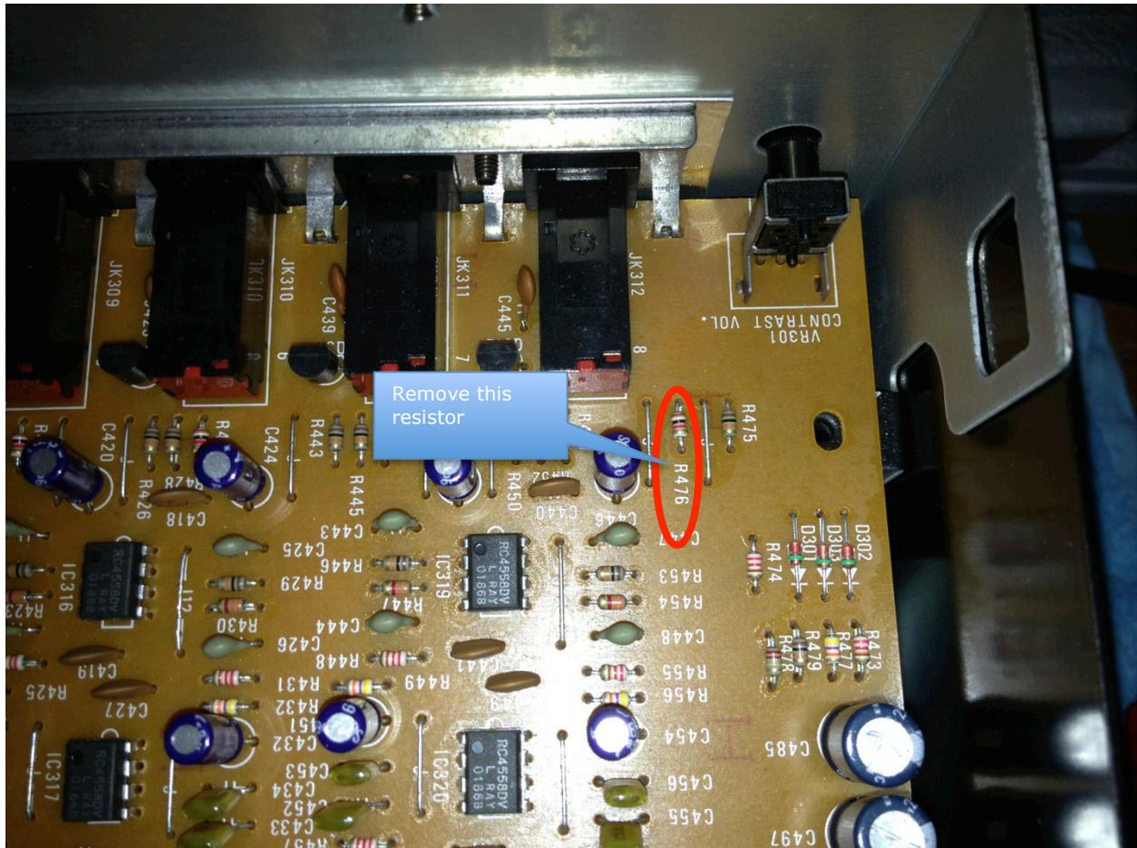
Rather than try different resistor values (and so need a whole load of resistors!), I elected to use a multi-turn trimmer (variable resistor) with a value of 10K. I snipped the 3<sup>rd</sup> leg off and formed the other two to fit the lead spacing of R476.
