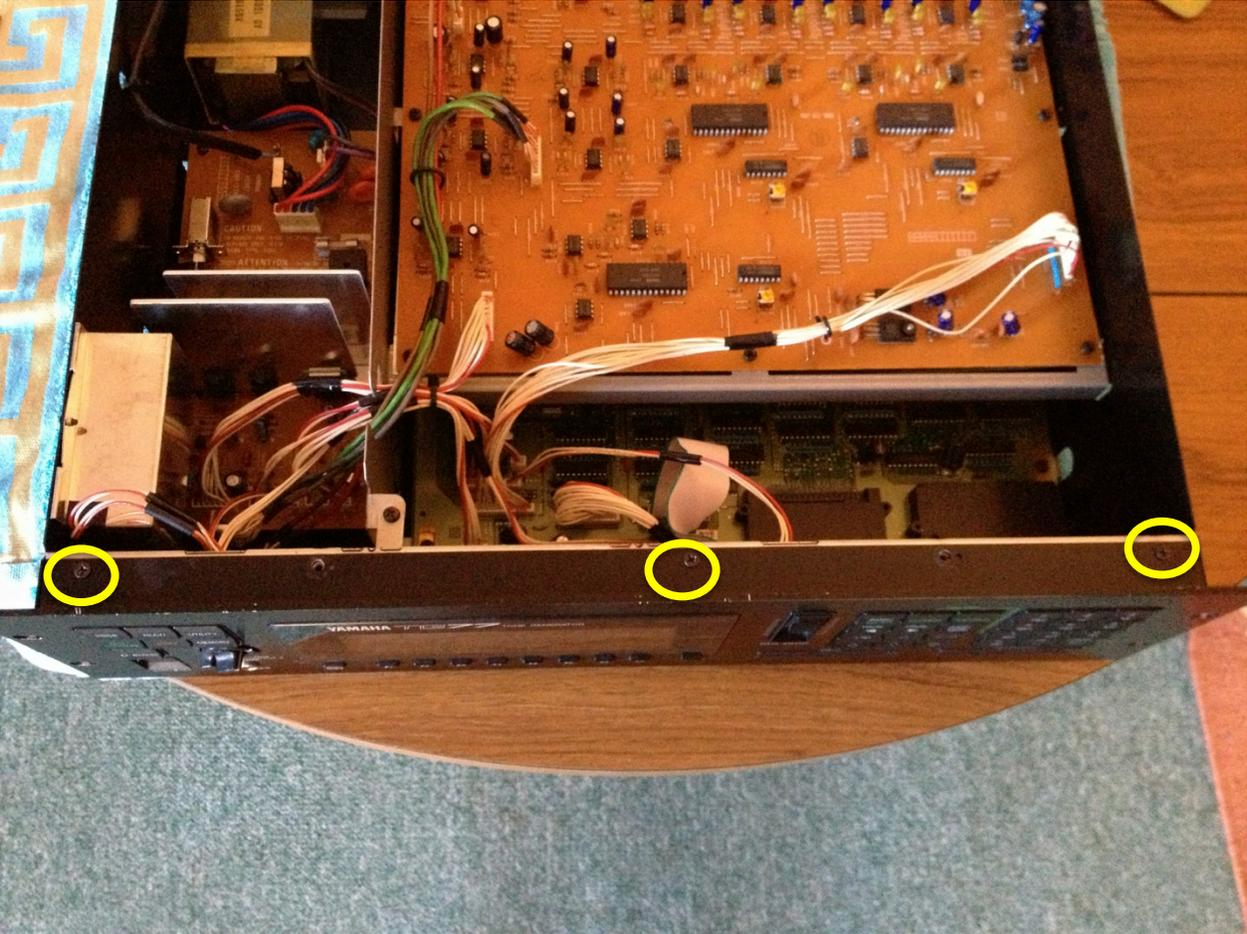
Now there are three more screws to remove at the base of the panel on the inside of the rack. They are a little hard to spot.
