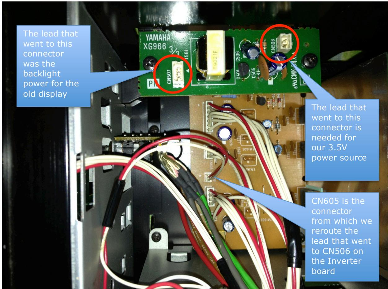
So remove the connector and wires running from the PSU to CN506 on the X6966 board. This board is now unpowered and no longer needed. It can be removed or left in situ. I elected to leave it in place as it's doing no harm (and no longer whining).
