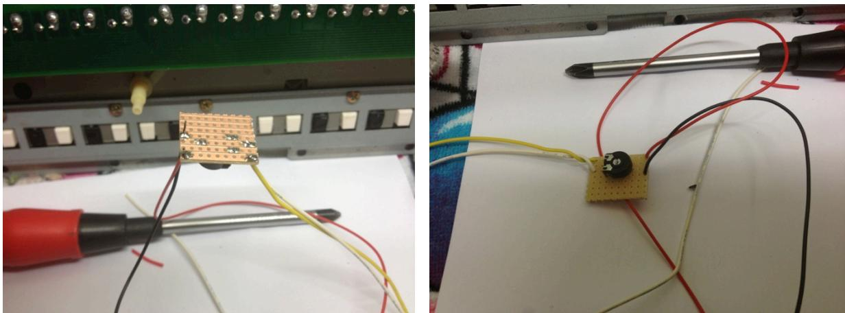
And this is where I placed it on the DM1 board (over to the left, not far from the edge of the board), using some sticky Velcro pads. I placed it here, as I wanted it in an accessible location so that I could adjust it in future if needed without having to disassemble everything!
