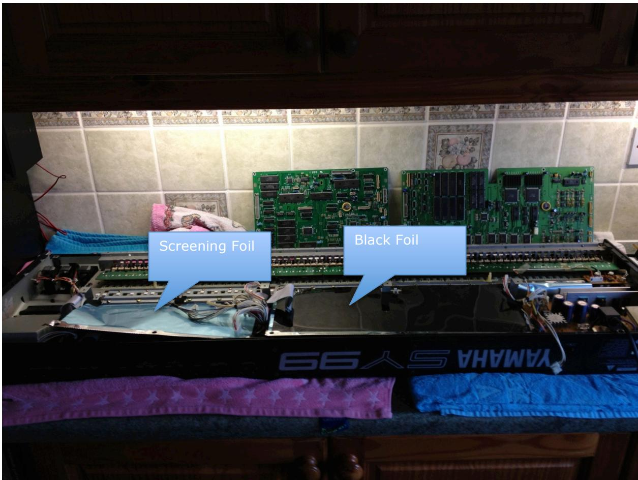
Removing the boards reveals screening material, which also needs to be removed. The black plastic under the DM2 board is easily removed, just note how it slots in the frame at the front of the keyboard.
