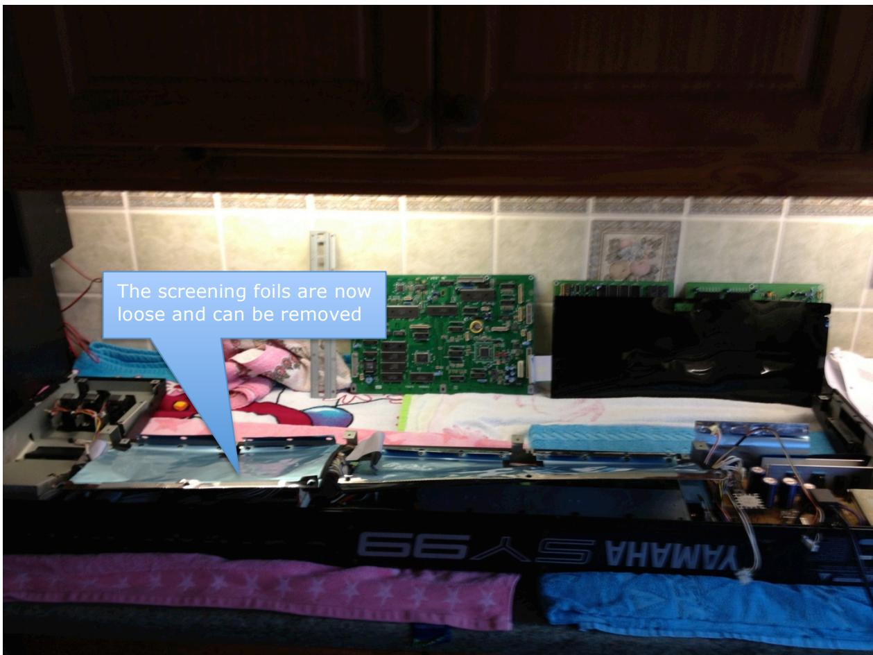
With the keyboard removed, the screening can now be removed, which will reveal the next layer!
