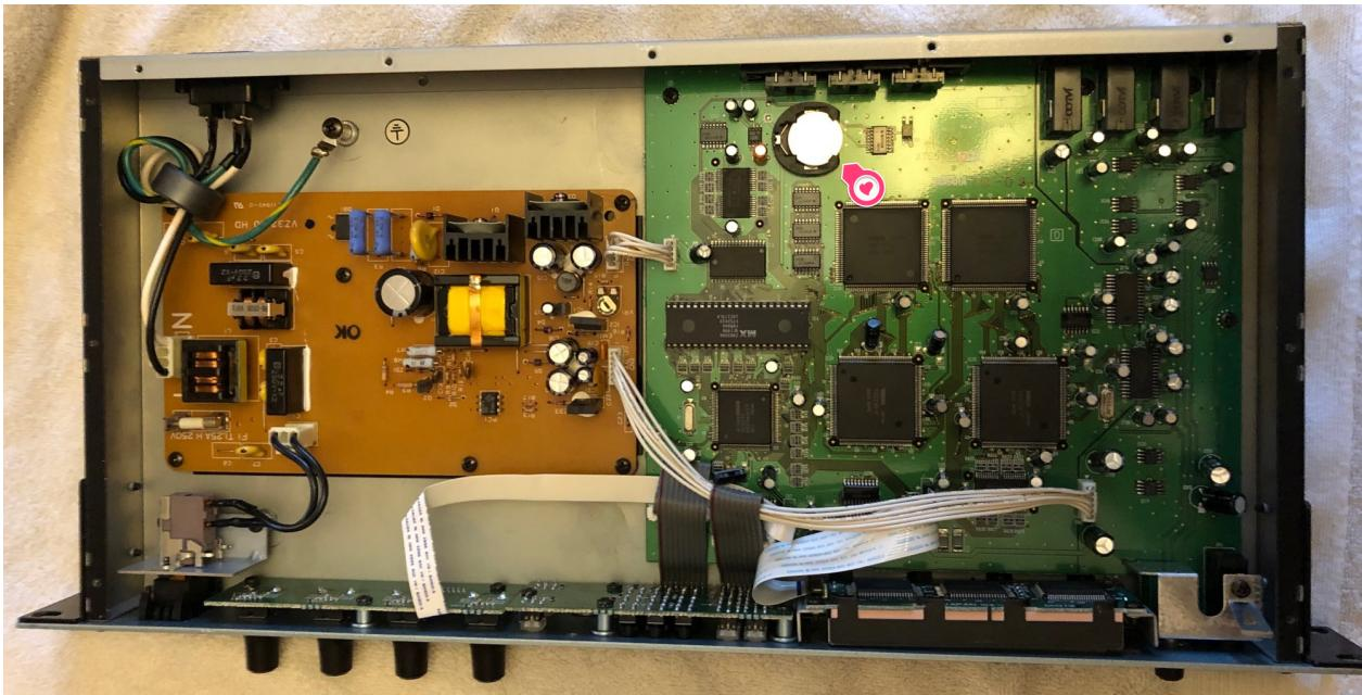
Before removing the battery, ensure that the other one is ready. Some batteries now come with a self-adhesive warning sticker that needs removing first, so you want to remove that if present, otherwise the circuit will not be made!
