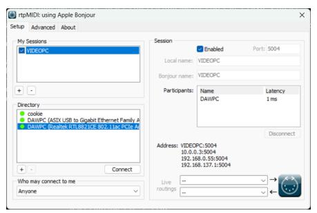
It's as simple as that, and RtPMIDI is fantastic at connecting two computers using MIDI with no need for additional MIDI hardware, although as mentioned above I find that a cheap network switch absolutely guaranteed successful network connection, certainly with my older dual laptop setup, and when I upgraded my rig I kept the network switch in the setup.
