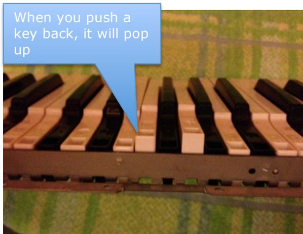
Once the key is loose, lift it up and pull it back towards the front, gently maneuvering it through the gaps at the front of the keybed.
